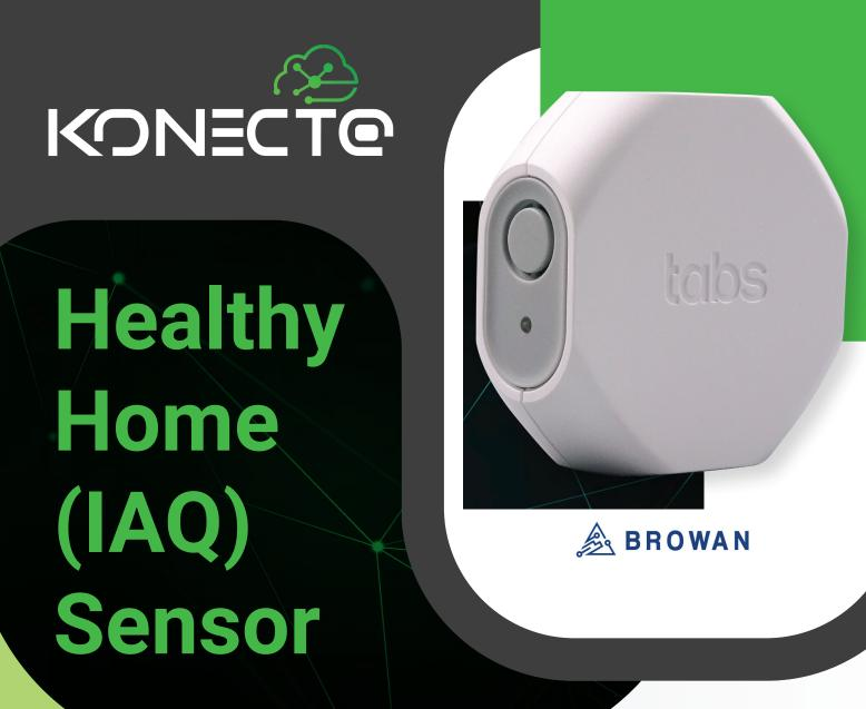
The Tabs Healthy Home sensor utilizes LoRaWAN connectivity to communicate the Temperature, Relative Humidity and Volatile Organic Compound levels of the surrounding environment. The intended use is to place the sensor within a room to determine if the air quality, temperature, and humidity are ideal.
