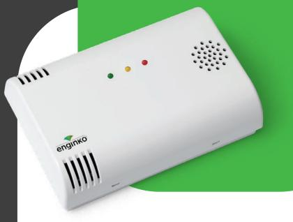
This device reads temperature, humidity, pressure, light intensity, air quality (expressed as IAQ or bVOC value) and CO2 and sends collected data over the LoRaWAN® network. 3 traffic light LEDs for air quality display with adjustable brightness. Ideally suited for a wide range of applications such as building automation, condition monitoring, predictive maintenance, security, healthcare and many more use cases.
